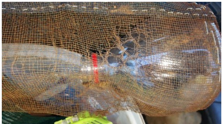
Fig 5. Damage inflicted to the enamelled steel mesh of a double-sided funnel trap by a large solifuge (Solifugae). Phinda Private Game Reserve, KwaZulu-Natal Province, South Africa, 2017. Photo: P.R. Jordaan.
